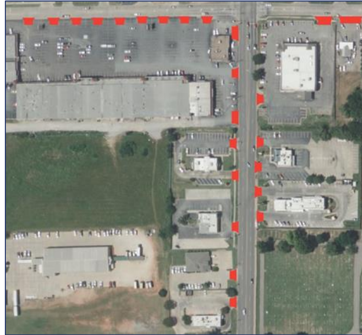
Example of Problematic Access Management
