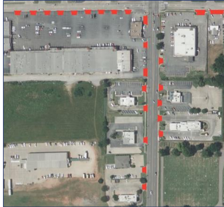
Example of Problematic Access Management
