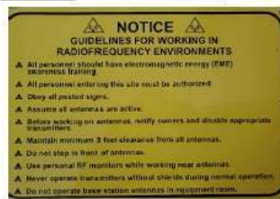
1 NOTICE - RF SIGN (BLUE) 12" x 18" DIGITAL PRINT MOUNTED TO 0.40 THICK ALUMINUM (OPERATIONS PROVIDED)
